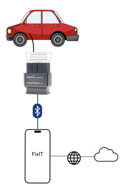
**OBD-II Dongle**: This small device plugs into the car's OBD-II port, which is typically found under the dashboard. The OBD-II dongle reads diagnostic data, such as trouble codes, directly from the car's onboard computer. These codes are generated whenever there is a problem, like an engine issue or sensor fault.
