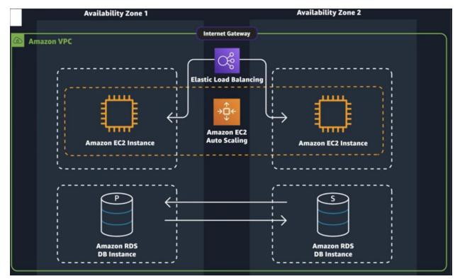
This architecture implements a highly available, auto-scaling application infrastructure deployed across two AWS Availability Zones (AZs) within a single Virtual Private Cloud (VPC). The design follows AWS best practices for fault tolerance and scalability.
